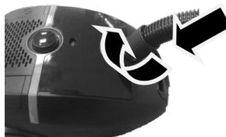
Remove the hose: Press the adaptors at both side of the hose end and then pull it out.
